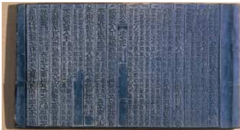
Engraved wooden plate, engraved on both sides, used to print the third and fourth folios of book 5 of the Major Commentaries on the Interviews of Confucius .
